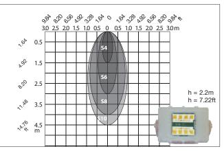
Detection area vs Sensitivity value (vertical angle 45°).
