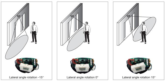
Adjust the lateral position to obtain the desired lateral angle sensing field.
