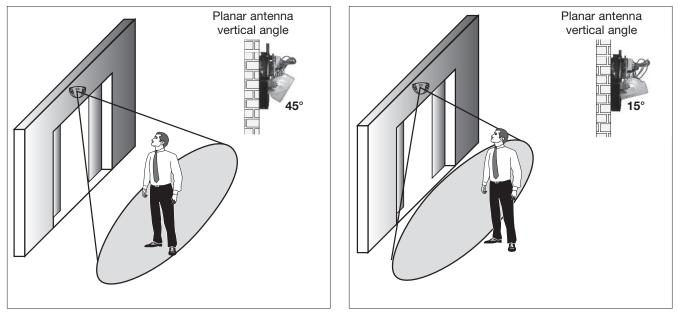
Adjust the vertical position to obtain the vertical sensing field close or far from the door.
