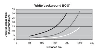
In this mode the maximum operating frequency is set to 250 Hz and detection is optimized for objects close to the background for top performance in general industry automation applications such as pallet wrapping machines, airport baggage conveyors, wood planks handling/stacking.
