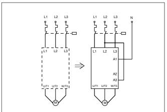
Fig. 2 For voltages higher than 480 VAC
