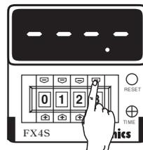
※ Set the position of decimal point using +, - buttons of digital switch.
