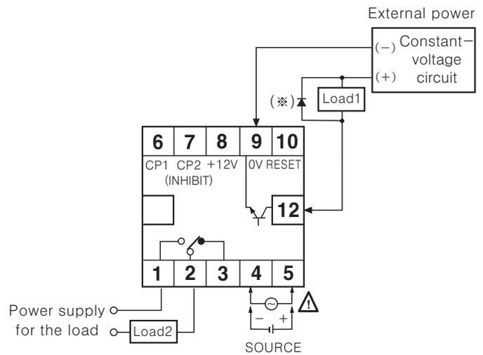
● (※) Please select proper capacity of load, because total current consumption should not exceed current capacity. (Max. 50mA)
