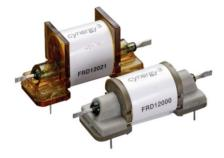
An open frame RF reed relay with 8kV isolation and 6A (at 30MHz) carry current, the FRD12000 series has been used many HF radio system specifications over the years, with applications in commercial maritime (GMDSS) equipment and military HF radio units worldwide. The use of vacuum reed switches with rhodium contacts offers high isolation voltages, low contact resistance and long operating lifetime.
